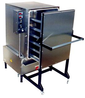
Steam boiling chamber UNIPAR U3-E is member of UNIPAR chambers and it is pressure free boiling device with *electrical heating*, controlled by adjustable time and temperature inside the chamber, with automatic water refilling.
