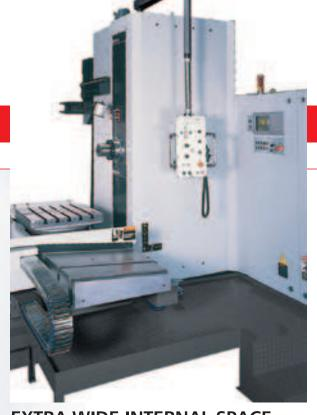
**EXTRA WIDE INTERNAL SPACE** It provides convenient loading and unloading for big workpieces.
