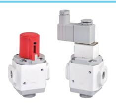
Shutoff valve is an easy and inexpensive way to add shutoff capability to an FRL unit. It allows the air supply to be closed and MVHR models can be operated either manually or by a solenoid valve. When the supply is closed, the compressed air is exhausted from the circuit behind the valve. Both positions of the manually operated model can be locked (padlock not included), which will contribute to safety during maintenance or adjustment. The valve is designed to be assembled
