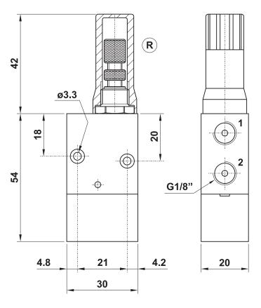
Notice: dimensions are the same for both valves - valve for signal start delay and valve for shorten the signal length.
