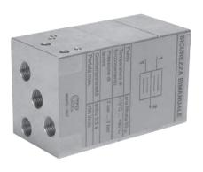
This valve is used to pilot high-flow directional control valves connected to machines which have a high risk of injuries to the hands. The machine operator must simultaneously operate, in a safe area, two three-way manual valves for correct operation. The safety valve will ignore a single depression of one of the manual valves. To repeat the cycle both pilot signals must be exhausted and the manual valves simultaneously actuated again.
