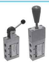
Lever valves are actuated by 120° lever turning. Both positions are detent. Draw bar valves are actuated by pressing the draw bar. Return to starting position is by pulling of draw bar. If the draw bar is during pulling out rotated to right, the force which is need for overcome the detent will be lower. Draw bar valves can be produced from stainless steel on request.
