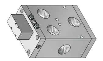
High flow valve series with flow capacity up to 28 000 Nl/min is suitable for fast air supply of big appliances, or higher quantity of appliances which are supplied from common distribution. Valves are pilot operated, using smaller, standard pneumatic actuated valves ISO 5599/1. These pilot valves are designed for external supply of compressed air, however the common supply is possible, but in this case, please contact our technical dept.
