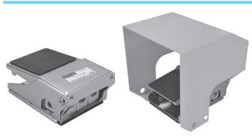
Valves without or with protecting cover are available with 3/2 and 4/2 function with or without detent.
