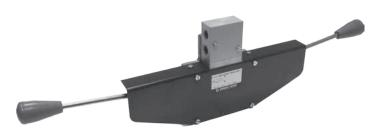
This safety valve is used in applications, where controlling by two hands at a time is necessary due to safety reasons (presses and etc.). Valve is actuated only when both levers are pressed together. If one lever will be pressed permanently, valve will not be actuated when the second lever will be pressed.
