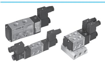
The popular valve series, which replaces valves series L and J. The basic usable features are kept and brings some improvements such as lower wattage, comparable or bigger flow capacity and better accessibility. Valves are solenoid pilot actuated. The product range covers functions 5/2 single or double solenoid and 5/3 with centre closed and exhaust position and position with pressure centre. Connector and coil are included in delivery.
