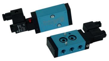
A range of indirectly operated valves with NAMUR connection (according to VDI/VDE 3845), based on our popular K-series valves. Available in 5/2 versions with one or two coils and 5/3 with a central position that is both vented and pressurized. A 3/2 version can be created using an adapter that is ordered separately. Using a connection plate, the valve can then be mounted directly on the cylinder inlet. A connector, sealings and screws are also included.
