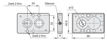
Connection plate for mounting the valve on cylinder inlet:
