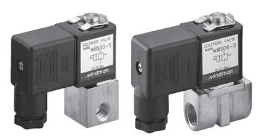
Direct solenoid actuated valve 2/2 normally closed with orifice 1 to 2.4 mm. The following sealing are available: NBR, EPDM and viton (teflon on request). Available fluid: air, inert gas, water, vacuum, oil, etc. Coil with Ex approval EExm II T4, or EEx ia II C T6 PTB are available on request.
