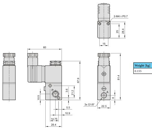
Dimensions of valve series MVDC with bracket
