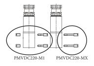
The screw sets are necessary for assembly the manifold of the valves. There are two sets available - set for first valve, which contains 2 nuts and 2 short screws and set for next valve, which contains 2 long screws - the required number of sets for next valves is about one set less than the total number of valves in the assembly (for example for 4 valves in manifold, 1 set of PMVDC220-M1 and 3 sets of PMVDC220-MX are required).
