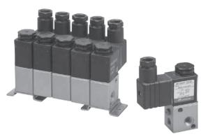
Small, direct actuated valve 3/2 or 2/2 normally closed with manual override. Valve can be used as a standalone or can be mounted together with other valves as manifold mounting. This manifold can be expanded at any time, valve and set of screws are required.
