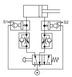
Cylinder is thrust, signal S1 is inactive, S2 is active.
