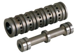
We make the spool and sleeve assembly from hardened stainless steel. The technical interest is that thanks to the precise grinding and honing of both parts, such accuracy is achieved that the piston in the sleeve moves on the air cushion. This essentially eliminates possible wear and at the same time the piston can be moved very easily and very quickly. The clearance is so small that there are no leaks even without a seal.
