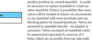
mounted to manifold directly - no adaptor is necessary. Valves mounted on manifold could be unmounted separately by unscrew of 2 bolts, which are accessible from top side (side with ports 2 and 4 of valves). Each separate coil must be wired with separate electrical cable. Or
