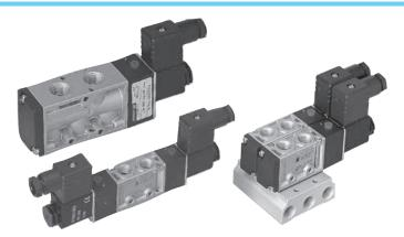
The popular valve series, which replaces valves series L and J. The basic usable features are kept and brings some improvements such as lower wattage, comparable or bigger flow capacity and better accessibility. Valves are solenoid pilot actuated. The product range covers functions 5/2 single or double solenoid and 5/3 with centre closed and exhaust position and position with pressure centre. Connector and coil are included in delivery.
