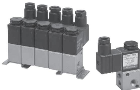
Small, direct actuated valve 3/2 or 2/2 normally closed with manual override. Valve can be used as a standalone or can be mounted together with other valves as manifold mounting. This manifold can be expanded at any time, valve and set of screws are required.
