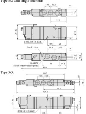
5x G1/8\* (valves with threaded ports) 53.7 Dimensions of valve series MVSY 188
