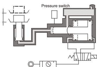
Booster can be used for short stroke hydraulic cylinders, for which is volume discharged by booster sufficient. In this case, any 5/2 valve can be used for control of booster and hydraulic cylinder, which copy the movement of booster.
